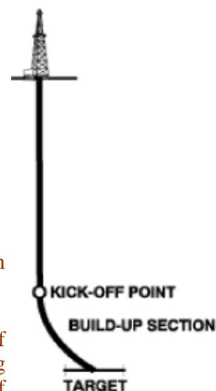
**Figure 2.4.18** : Deep kick-off and build trajectory
