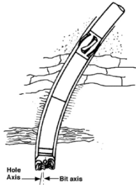
Figure 2.4.57 : One possible interpretation of the pendulum effect
