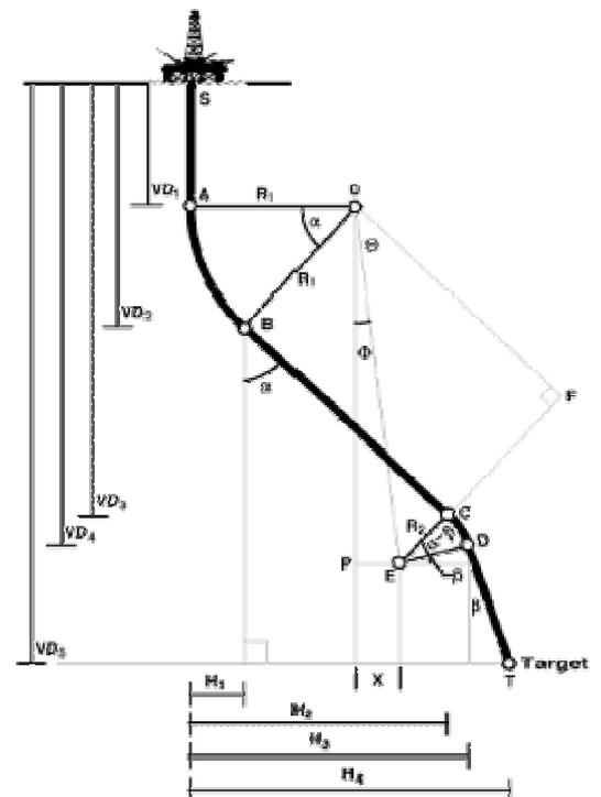
Figure 2.4.79 : Cross section through an S-type well
