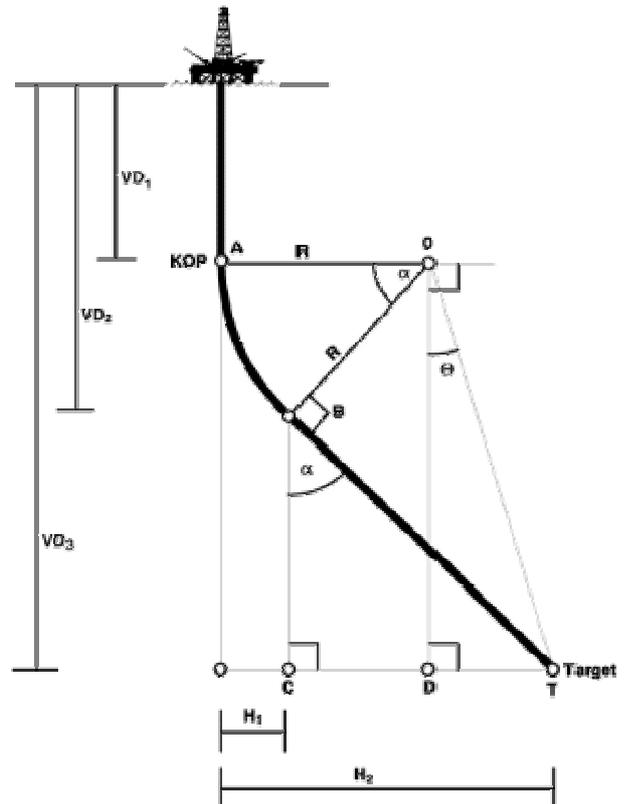
**Figure 2.4.78** : Cross section through a "build and hold" type well
